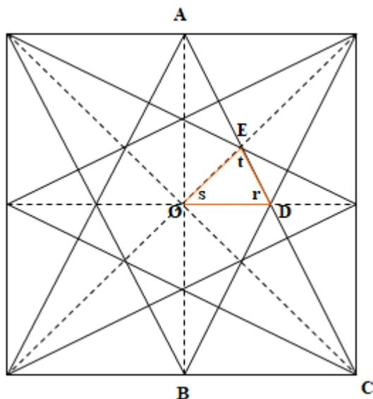
The tile has four axes of symmetry. Hence all eight sides of the octagon are equal. Length of each side of the square is 1 foot.
